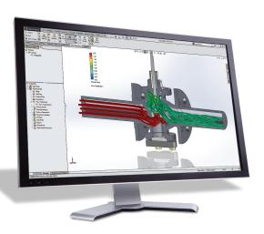
Flow Simulation's exclusive Turbulence Model means that laminar, transitional, and turbulent flow regimes are automatically determined with no need to specify flow characteristics. The ability to directly model flow regimes eliminates the need for a CFD specialist. The turbulence model also offers shorter setup times and increased model accuracy compared to traditional approaches.
